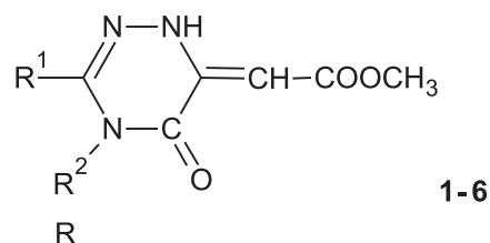
Figure 1. Structure of methyl 2-[5-oxo-3,4-di-substituted-1,4,5,6-tetrahydro-1,2,4-triazine-6-ylidene]acetate derivatives
