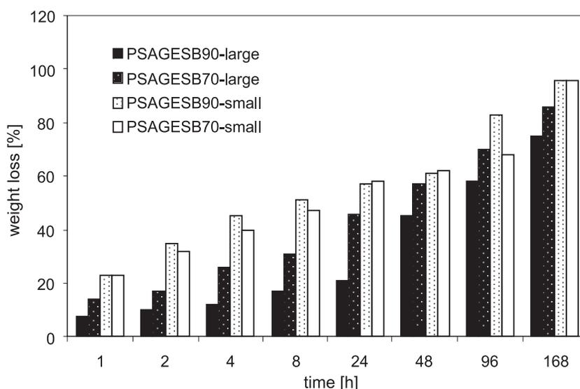
Figure 4. Effect of polymer composition and size of microparticles on the hydrolytic degradation of blank microspheres in PBS at 37°C
