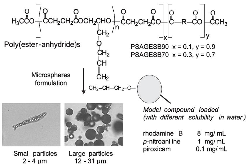
Figure 1. The scheme of preparation of model compounds loaded poly(ester-anhydride) microspheres
