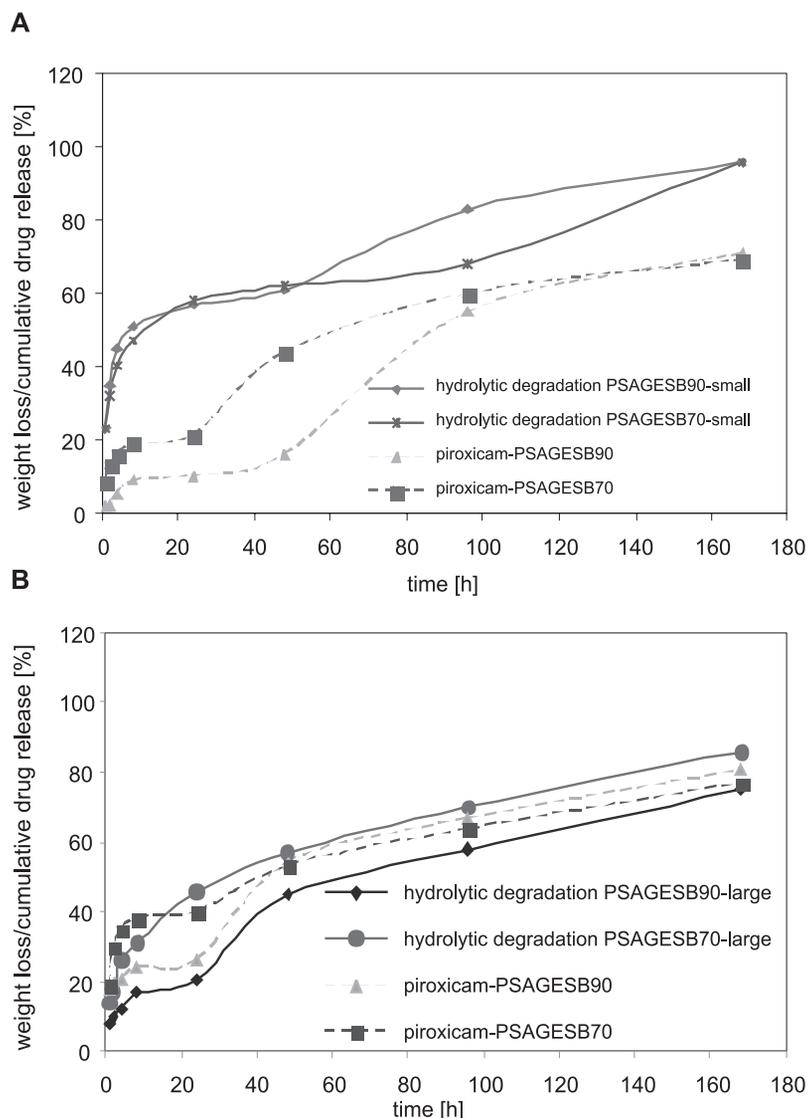
Figure 9. The comparison the release profiles of piroxicam with hydrolytic degradation of small (A) and large (B) microspheres
