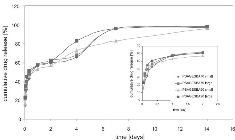
Figure 6. Cumulative release profiles of *p*-nitroaniline from various microspheres as a function of time
