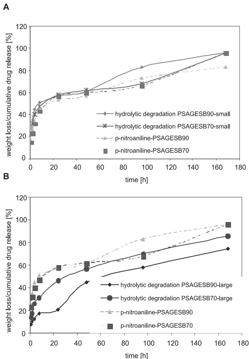
Figure 8. The comparison the release profiles of *p*-nitroaniline with hydrolytic degradation of small (A) and large (B) microspheres
