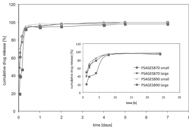
Figure 5. Cumulative release profiles of rhodamine B from various microspheres as a function of time
