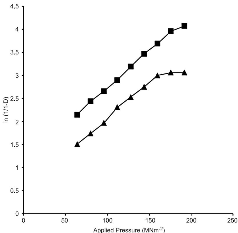
Figure 3. Heckel plots for tablets made from the gums. ■ NMG, ▲ ACA
