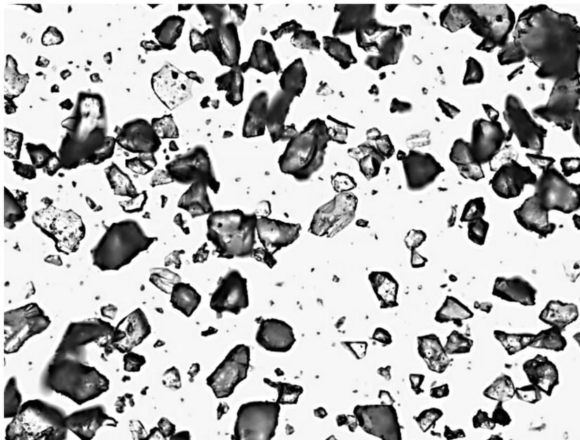
Figure 1. Photomicrograph of neem gum powder (100x)
