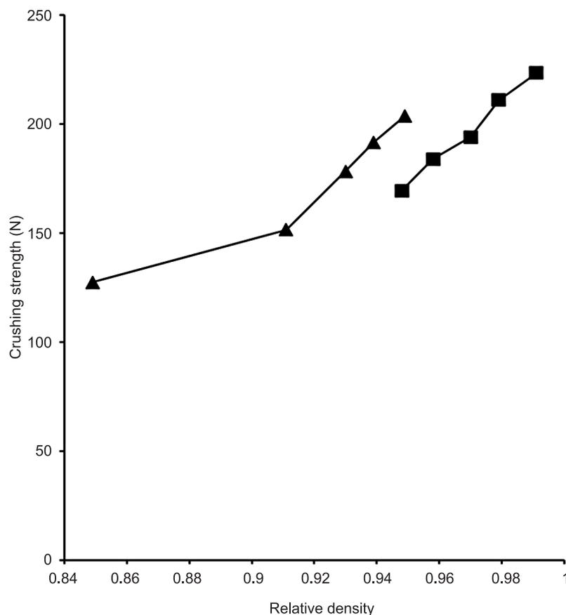
Figure 6. Plot of crushing strength *versus* relative density for gum tablets. ■ NMG, ▲ ACA
