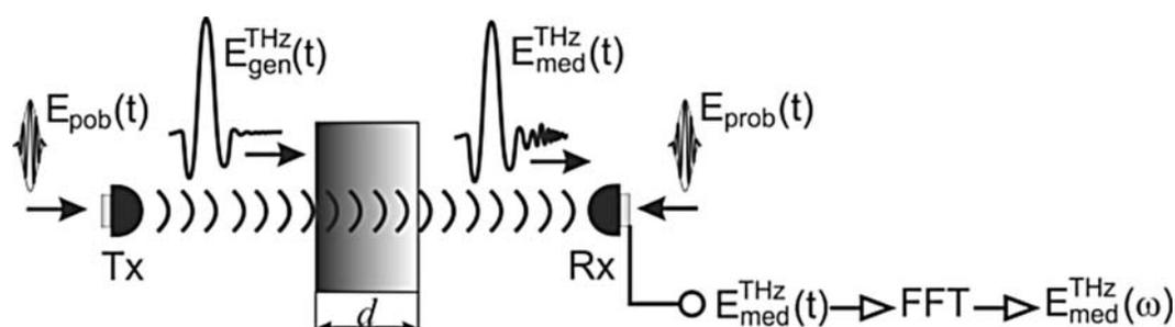
Figure 2. Coherent homodyne detection – the measuring and calculations of the signal with the sample, where  $d$  – thickness of the sample. FFT – Fast Fourier Transform operation on the measured signal
