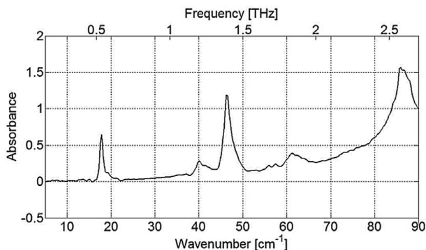
Figure 6. Terahertz spectrum of lactose monohydrate
