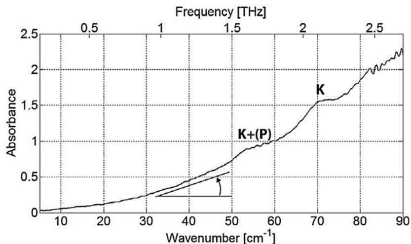
Figure 14. Terahertz spectrum for mixture of Pluronic F127 and ketoconazole in the weight ratio of 50/50. K - contribution of ketoconazole, (P) - weak contribution of Pluronic. The angle of the slope is indicated (explanation in the text)
